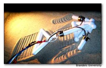
A computer-designed and automatically built "arrow" robot crawls through the sand. Its symmetric shape arose after hundreds of generations' worth of simulated evolution.
