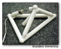
The 3-D printer, also known as a plotter or milling machine, could create the complete robot, joints and all, within its 8-by-8-by-12-inch parameters. All the humans had to do was snap in the motors and hook the robots up to their electronic
